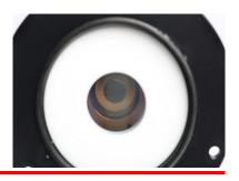
For low light-level applications, such as the measurement of spectral irradiance, the photomultiplier is an indispensable spectroradiometer component. The DH-3 photomultiplier, consisting of a housed end-window multi alkali (S20 photocathode) is the detector of choice for such measurements over the UV-Visible region.
